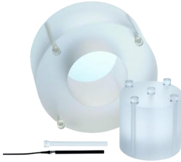
Figure-5.1: Cylindrical PMMA Phantom used at INMP, AERE, Savar, Dhaka
