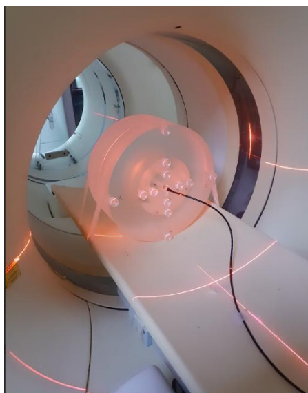
Figure-5.2: CTDI measurement using Phantom
