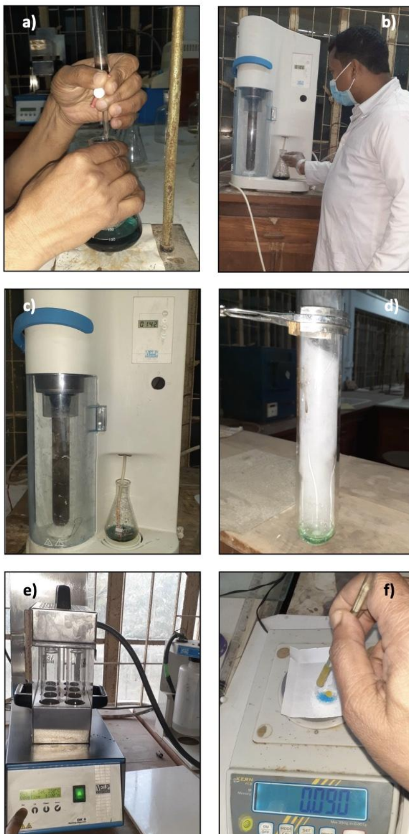
Photo 7.5 Determination of chemical composition of ostrich egg: a) titration of yolk protein; b) distillation of protein; c) distillation plant for protein; d) digested yolk after Kjeldal digestion; e) Kjeldel digestion and f) measuring of yolk
