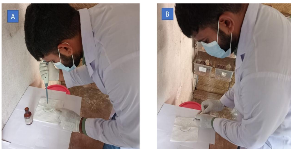
Photo 3.2: Preparation of working solution. A) Taking DEHP solution by using micro-pipette B) Withdraw working solution by feeding needle.
