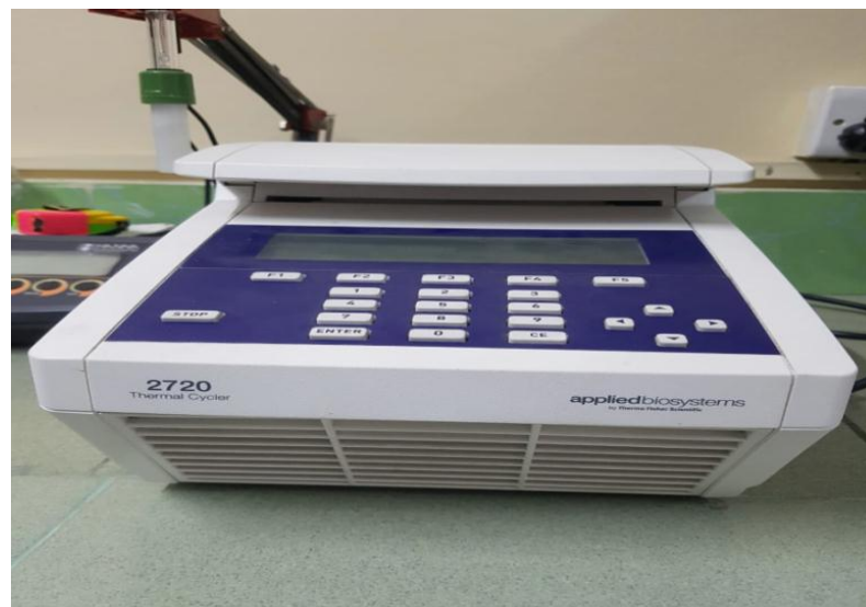
Plate 34: Conventional PCR model ABIS 2720
