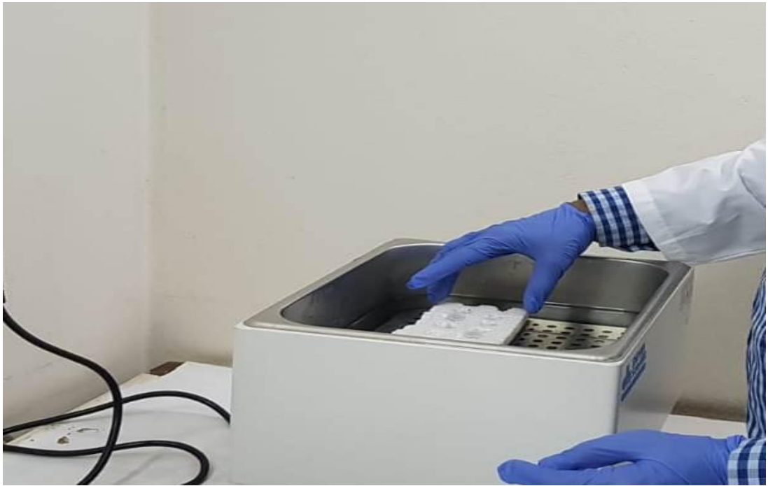
Plate 21: Incubation of homogenates at 55°C
