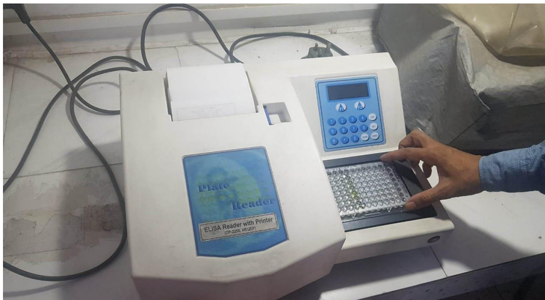
Plate 18: Taking reading by ELISA reader
