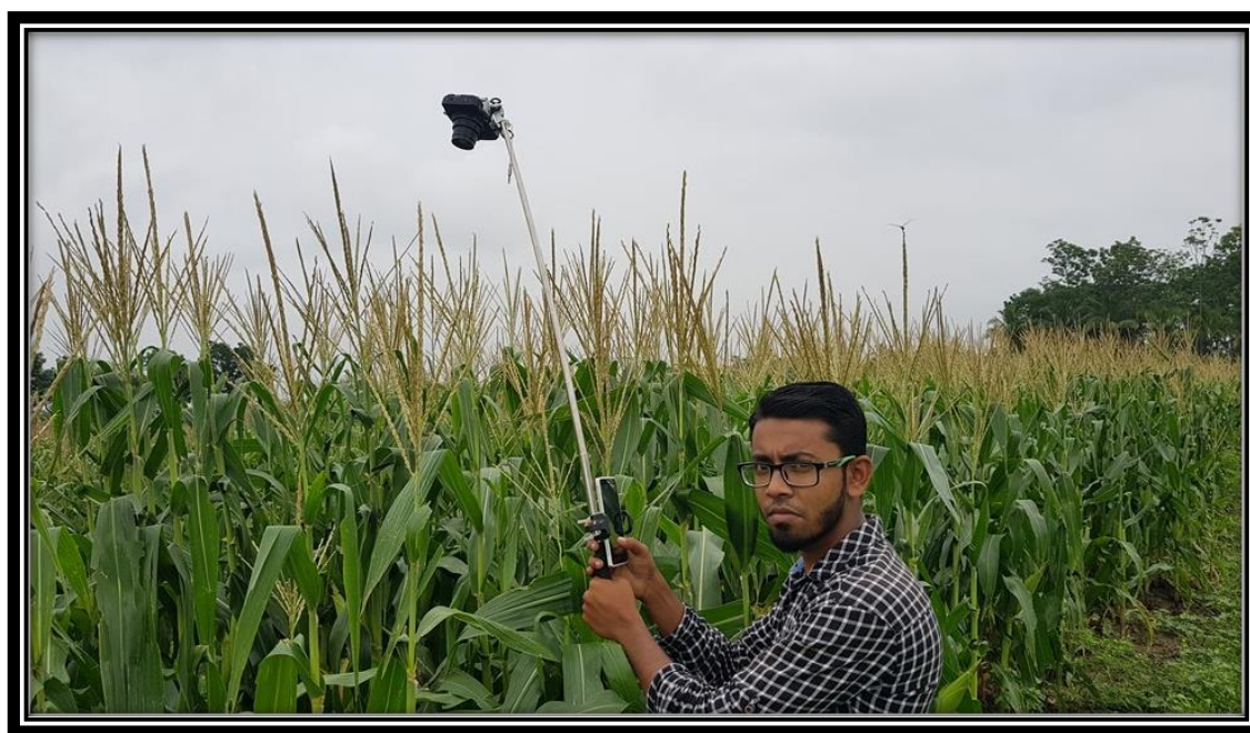
Plate 8: Modified selfie stick camera controlled by blue tooth connection with mobile phone
