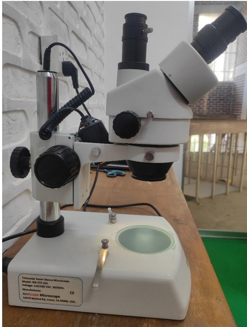
Plate 3. Trinocular Zoom Stereo Microscope (Model: SM-2TZ LED, AmScope Microscope, Irvine, CA 92606, USA) observing and counting egg and first instar larva
