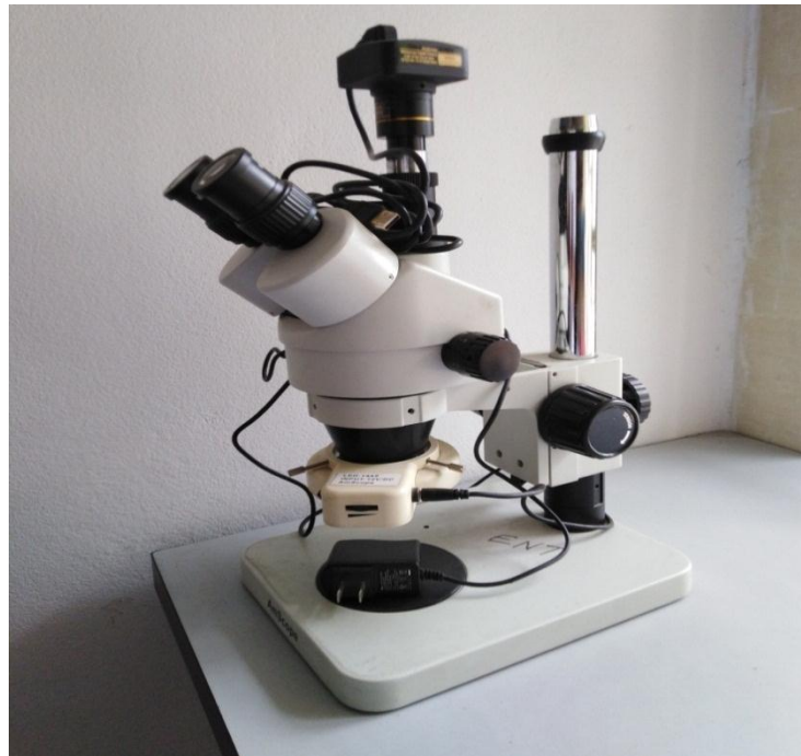
Plate 5. Stereo Microscope (Model: SM-2TZ LED, AmScope Microscope, Irvine, CA 92606, USA) for observing different stages and counting eggs
