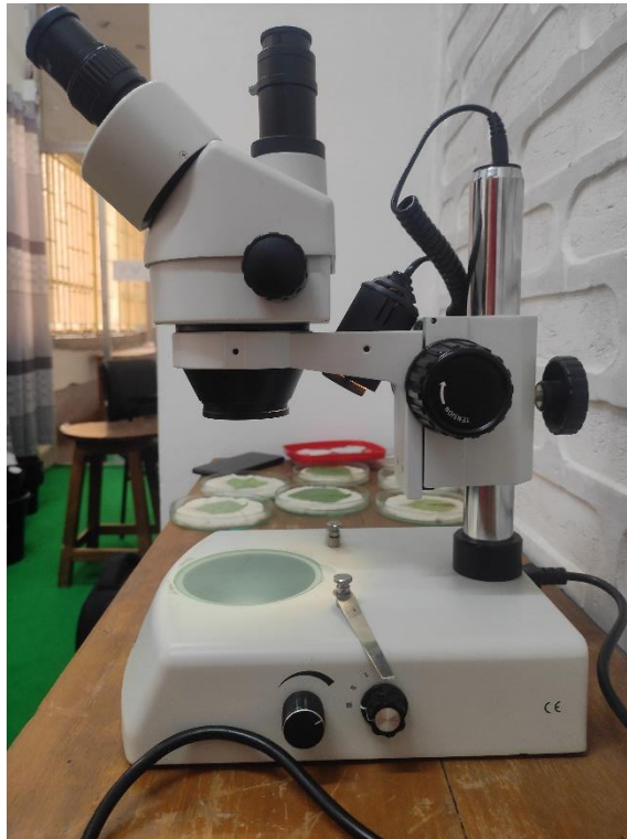
Plate -5: Stereo microscope (model: SM-2TZ LED, AmScope Microscope, Irvine, CA 92606, USA) for observing and counting egg and first instar larva of D. maculatus
