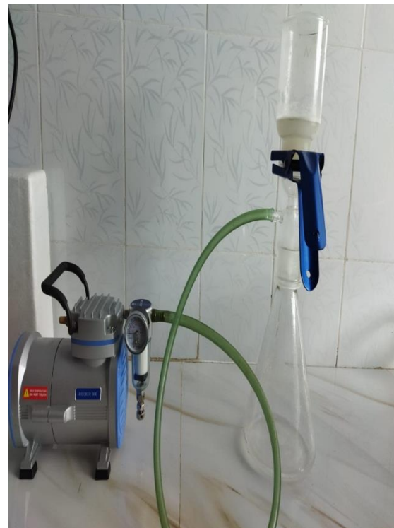
Figure 3.5 Filtration process of crab samples for microplastics identification
