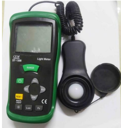
Figure 3.14: Light intensity measuring device.
