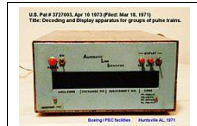
The first caller identification receiver (1971)
