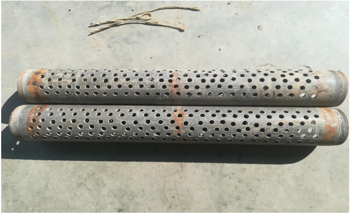
Figure 3.8: Perforated pipe (10 mm diameter)
