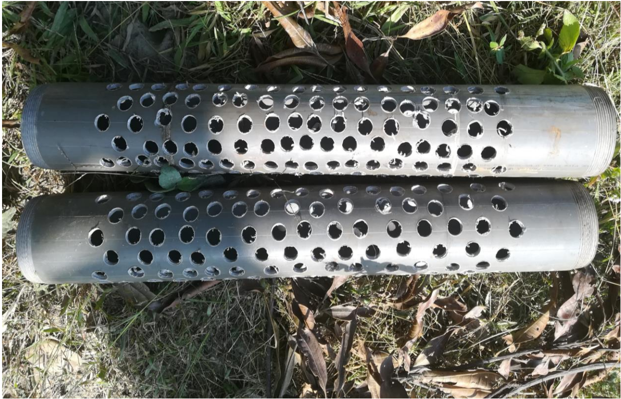
Figure 3.10: Perforated pipe (20 mm diameter)
