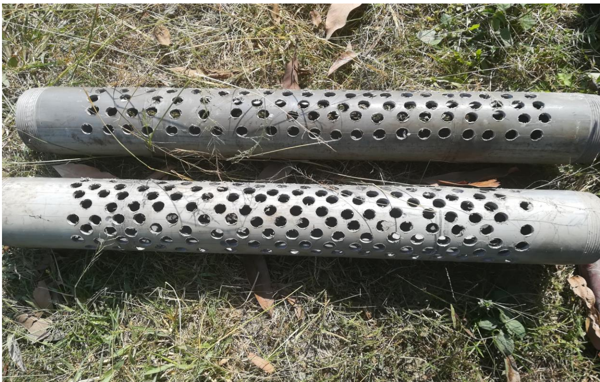
Figure 3.9: Perforated pipe (15 mm diameter)
