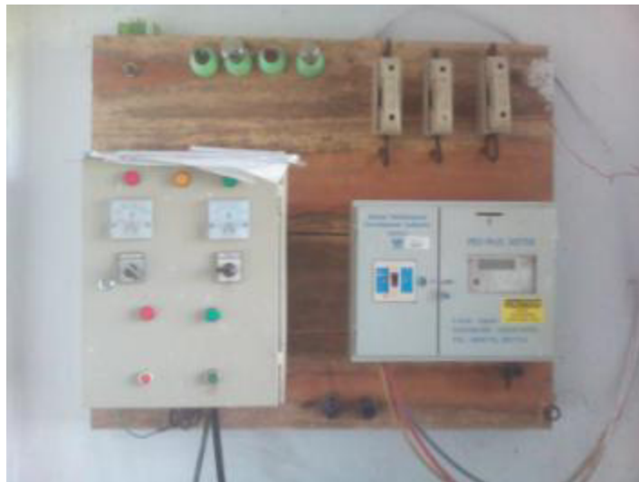
Figure 3.4: Prepaid meter board with Ameter and voltmeter
