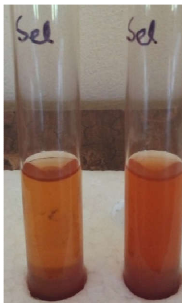
Plate 39: Selenite Broth test for E. coli showing positive result by the change of the medium to brick red colour (right) and control (left).
