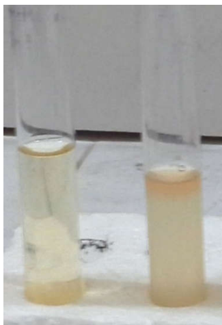
Plate 24: Voges-Proskauer test for Pseudomonas spp. showing negative result by no change of the medium (right) and control (left).
