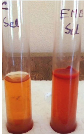
Plate 39: Selenite Broth test for E. coli showing positive result by the change of the medium to brick red colour (right) and control (left).
