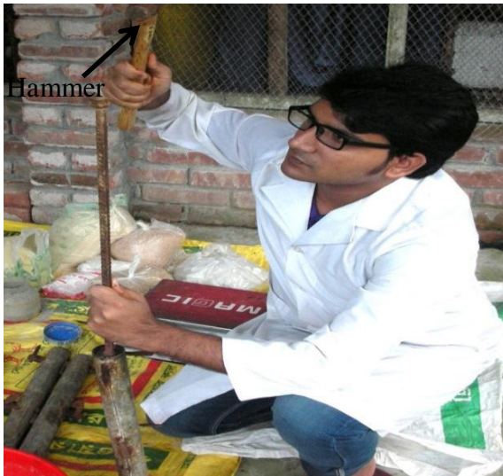
Photo 9. Hammering and tightening the UMMC tube screw to make a hard and compact UMMC
