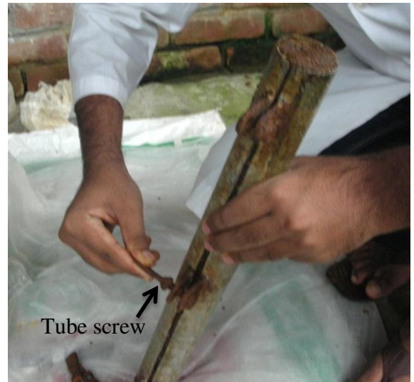
Photo 9. Hammering and tightening the UMMC tube screw to make a hard and compact UMMC
