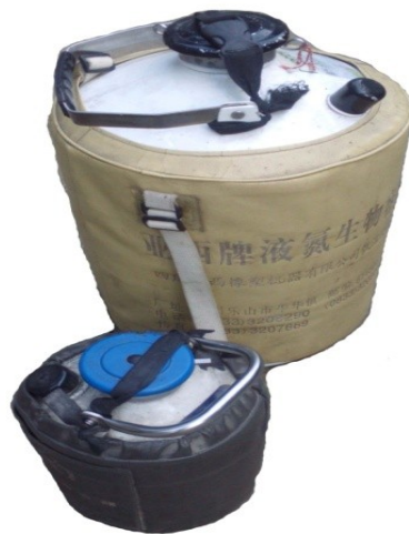
Fig.:1.1 Liquid Nitrogen Tank with Vacuum Insulation
