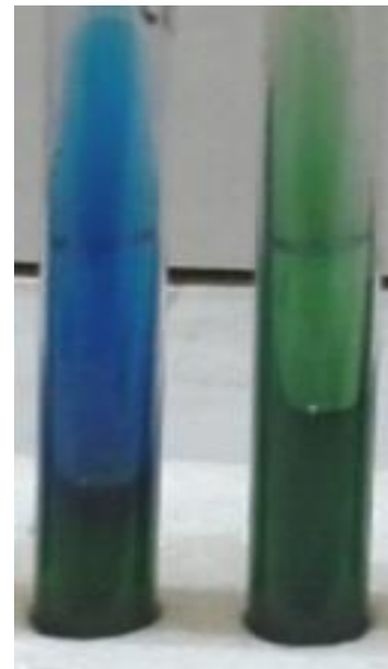
Plate. 47: Simmon's Citrate Test for Pseudomonas spp. showing positive result by colour change of the medium into blue colour (left) and control (right).
