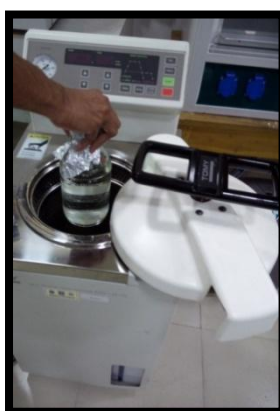
(B) PPS was placed in an autoclave for sterilization
