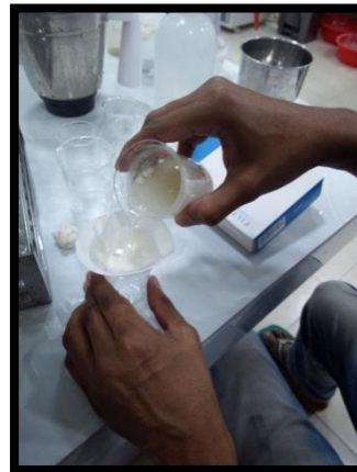
Plate: (B) Homogenized sample was filtered with a filter paper
