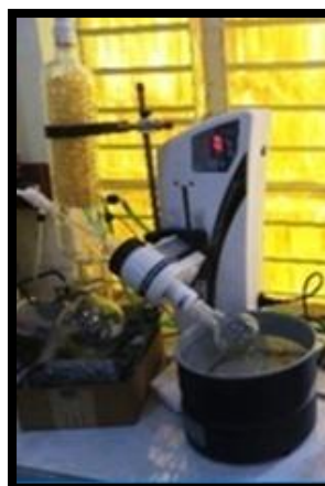
Plate: (B) Evaporation of fish oil was done in a rotary evaporator
