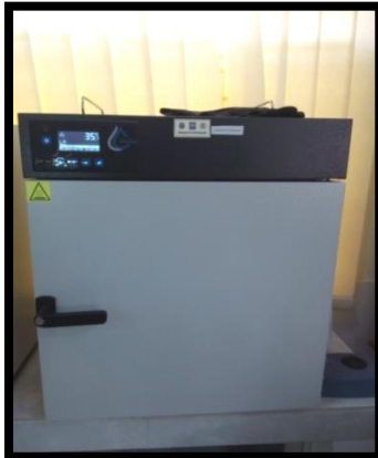
Plate: (A) Prepared plates were incubated at 35 0 C for 48 hrs in dry air oven
