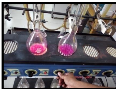
Plate: (C) Kjeldahl flasks were placed on the Kjeldahl apparatus
