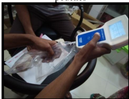
Plate: (C) Gas ratios of sealed packages were checked
