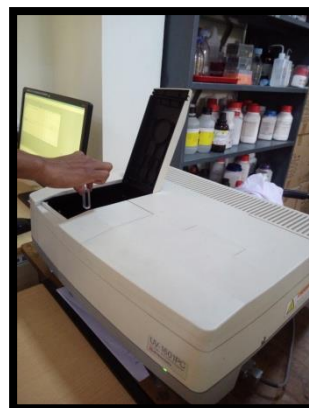
Plate: (D) Reactive substances absorbance were measured in spectrophotometer
