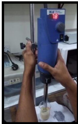
Plate: (A) Homogenized the fish sample in a homogenizer
