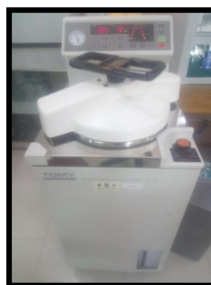
Plate: (C) Autoclaving was done for 15 min at 121°C
