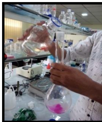
Plate: (B) Added 6.5 mL of 20% NaOH to the Kjeldahl flask
