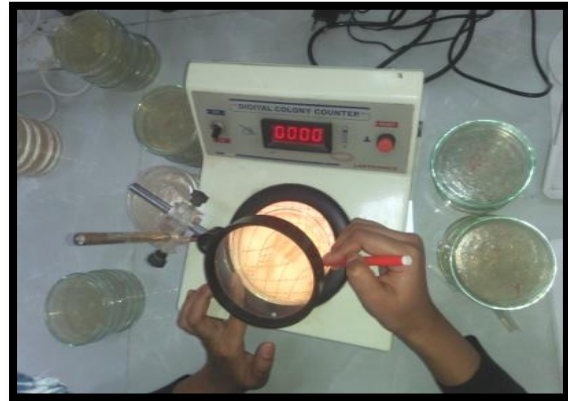
Plate: (B) Bacterial colony was counted in a digital colony counter
