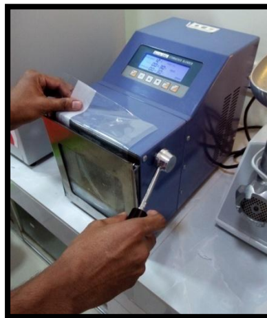
Plate: (B) Diluted sample was blended in a stomacher blender
