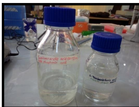
Plate 20: Some key chemicals used in the study, 20% trichloroacetic acid (in 2 M phosphoric acid) (on left) and 2- thiobarbituric acid (0.005 M in DD water) (on right) respectively
