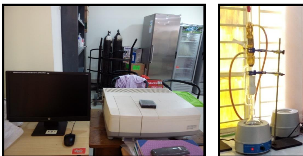
Plate 17: Showing PC connected spectrophotometer (on left) and Soxhlet apparatus (on right) respectively
