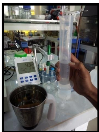
Plate: (A) 50ml of distilled water was added with 10 grams of sample
