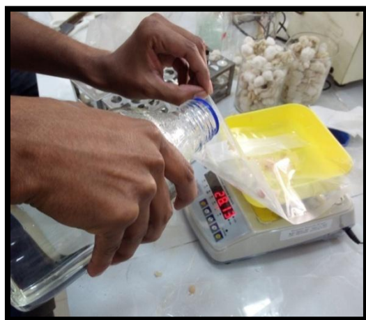
Plate: (A) Fish sample was diluted by adding PPS
