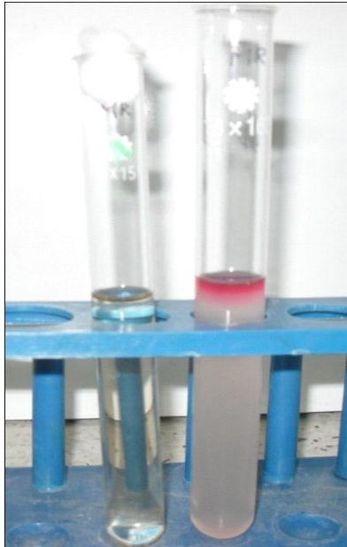
Plate 16: Methyl-Red test for E. coli showing the medium was changed to bright red color (right) and control (left).
