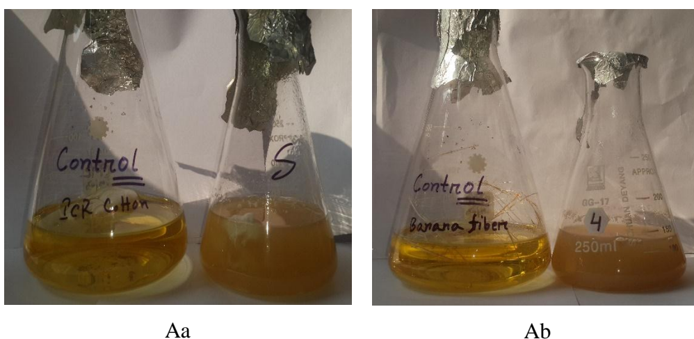
Fig 24: Sub fig (Aa and Ab) showing ICR cotton and banana fiber treated with consortium (HSTU-2, 3, 6, 7, 9 and 10) respectively along with their control. It is evident that compared to the control the treated fiber is showing a dense solution slightly proving that the bacteria have successfully removed some impurity in them.
