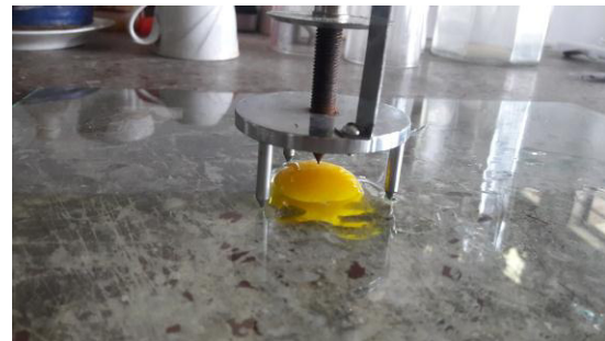
Diameter of egg albumin determination
