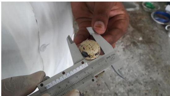
Egg width determination
