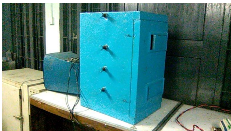
Fig 3.2: Multistoried universal cabinet dryer used for drying of spinach.
